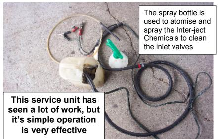
Organise a spray Bottle to be filled with Diesel Care & Cure Cleaner to be used later to help clean the inlet valves, as well as the Inlet manifold while the engine is running. Always engine the warm up to operating temperature before attempting this Service. especially the valve cleaning process.
